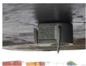
ENFORCER® KING PIN LOCK Prevents trailer theft
